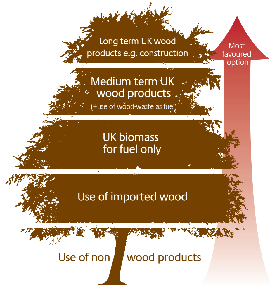
Figure 11: Hierarchy of wood uses by carbon impact
